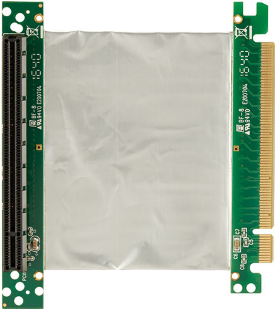
PClex16 to PClex16 riser card, L=100 mm
